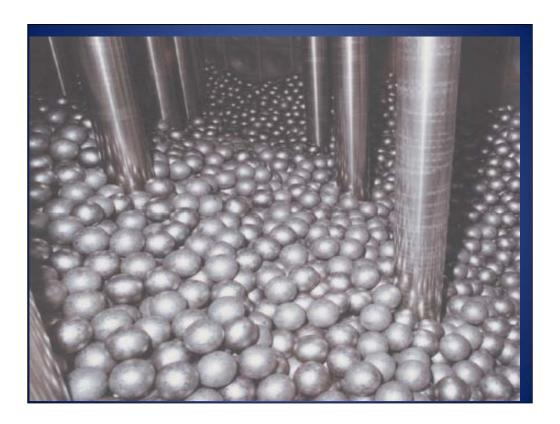
This photo depicts a collection of "TRISO" nuclear fuel elements in a Pebble Bed Modular Reactor. Each "pebble" is a collection of thousands of smaller spheres consisting of a core of nuclear fuel (e.g., uranium) surrounded by coatings of pyrolytic carbon, porous carbon, and silicon carbide; the pebbles observed here are about the size of a billiard ball. Such a plant is under construction in South Africa.
