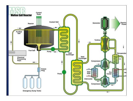
Another Generation IV reactor concept is depicted here, the Molten Salt Reactor. Again, higher efficiencies are to be gained from high temperature reactors in which water (used in the common water-cooled reactors of today) has been replaced
