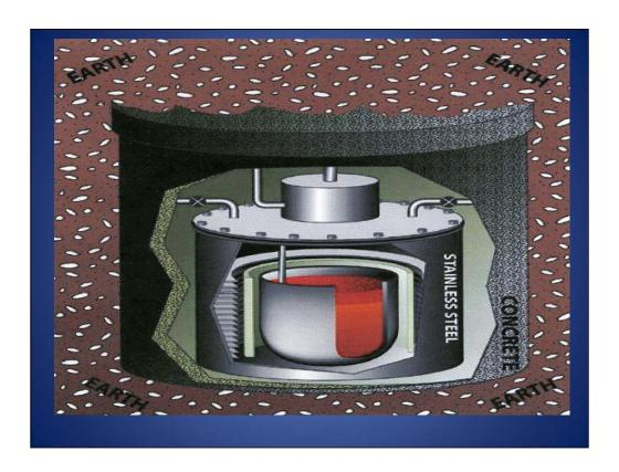
A new candidate for nuclear power is the "mini-reactor". Shown here is an artistic representation of the "Hyperion" version, invented by Otis Peterson of the Los Alamos National Laboratory. The unit can be shipped by truck, has no moving parts, and requires no operator. It produces ca. 70 MW of thermal energy (27 to 30 MWe), enough to power over 20,000 homes. It is inherently safe and proliferation-resistant. After five years, the unit can be refueled (uranium hydride).
