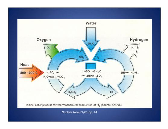
The process shown here is but one means of generating hydrogen with the use of a high-temperature reactor. Here, chemical catalysts H2SO4 and HI are used to produce hydrogen and oxygen from water.
