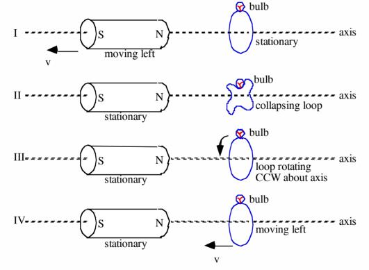
29. In which of the above figures will the light bulb be glowing?(a) I, III, IV(b) I, IV(c) I, II, IV(d) IV(e) None of
