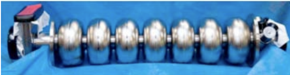
CEBAF-7-cell niobium elliptical cavity
