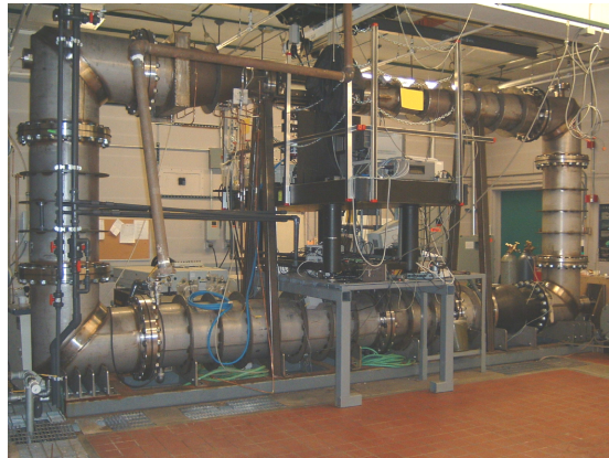
9- Inch Cavitation Tunnel at the University of Michigan
