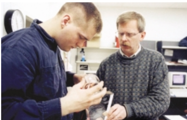
Figure 4.3. Research at an undergraduate institution. Hope College undergraduate Joe Bychowski works with Professor Paul DeYoung to prepare a light guide and photomultiplier tube for attachment to a long scintillating plastic bar for nuclear reaction studies with radioactive beams. When completed, this component will form part of a large-area wall of detectors.
