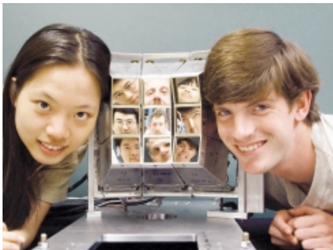
Figure 3.3. Reflections of the next generation. The Large Area Silicon Strip Array (LASSA) at NSCL reflects the images of several graduate and undergraduate students who were involved in its design and construction. The detector array comprises nine telescopes, each of which consists of a thin, 65- \mu\text{m} silicon-strip detector, followed by a thick, 1.5-mm silicon-strip detector, backed by four 6-cm-long CsI detectors. This detector is a working prototype for the next generation of experimental devices for use with rare isotope beams.
